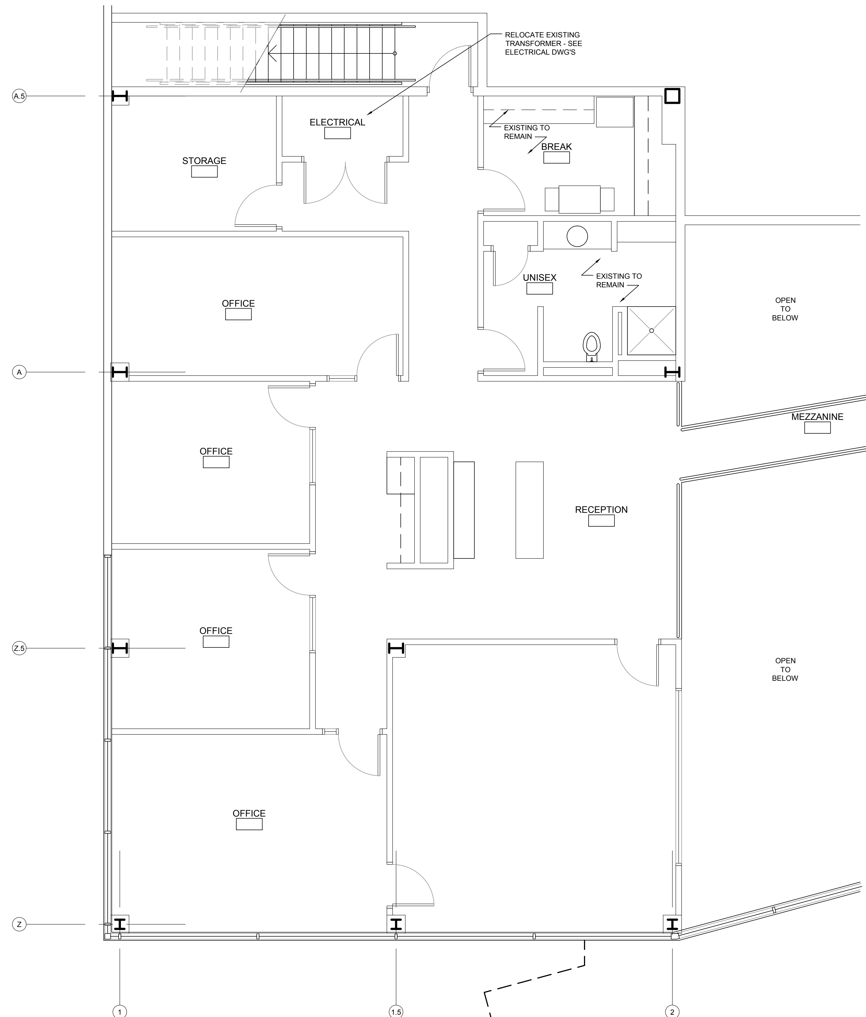
3 D-4 DEMOLITION PLAN - UPPER LEVEL (WEST) Scale: 1/4" = 1'-0"
